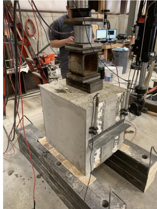
Figure 3. Connector shear test loading apparatus
